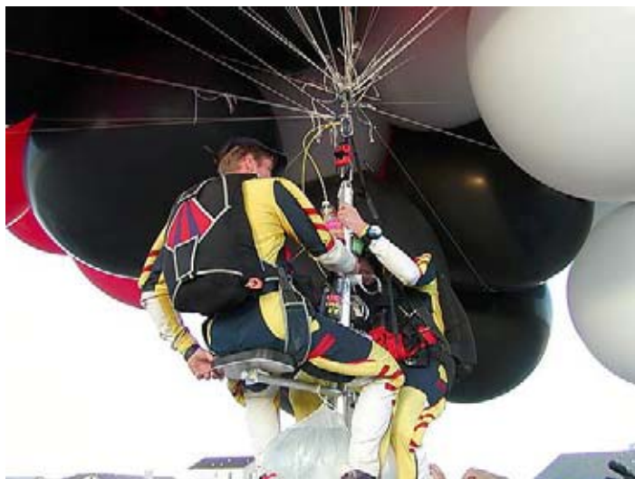
The teeter-totter. Note the water ballast below the seats.
